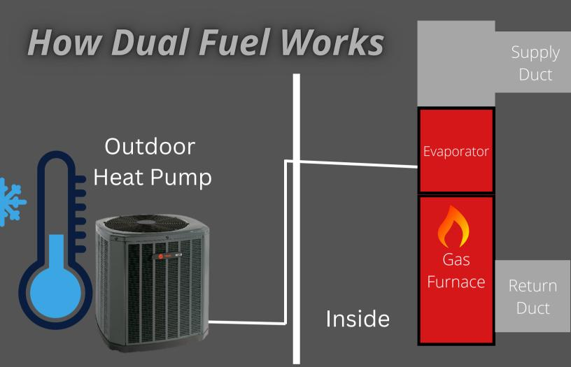
Dual fuel systems utilize two sources of energy for heating season. The two energy sources being gas and electricity. The heat pump system will heat your home using electricity during mildly cooler temperatures while more efficient for operation. As the temperature outdoors reaches cooler temperatures where the heat pump is not as efficient, the gas furnace will take over automatically to heat your home more efficiently.
